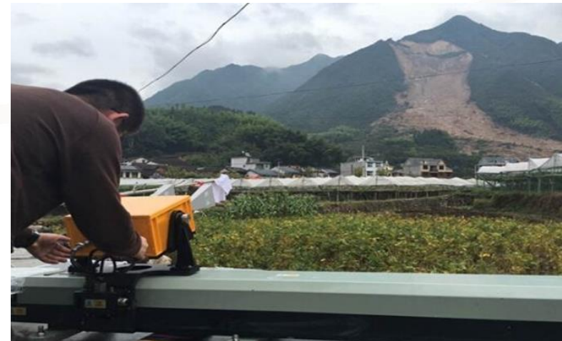
Radar displacement monitoring
